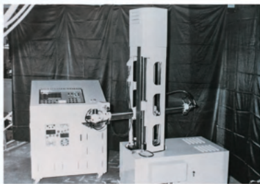
Aluminum die-casting operation robot
