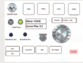
Displays screens created by TwinCAT3 HMI Web
