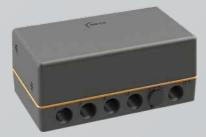
**RCB10+** is a 4-channel control box with a 2 Ah battery pack and an external charger, that can operate almost any actuator. By connecting the control system to a PC you can easily configure your individual settings. It has customizable current limits, soft
